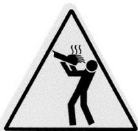
indicates the maximum height for containers with liquids. To avoid burns, do not put in the upper levels to the indication given by the symbol “products that can become liquid and can not be visible to the operator”
