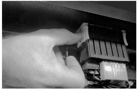
8. Push to release brackets for controller.
