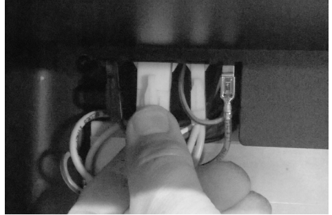
2. Dismantle the cables above the heating element and Fan box can be removed.
