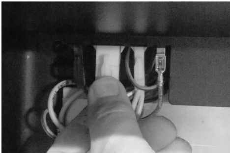
5. Dismantle the cables above the heating element.
