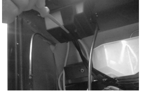
2. Place a screwdriver in cover, and pull to dismantle.
