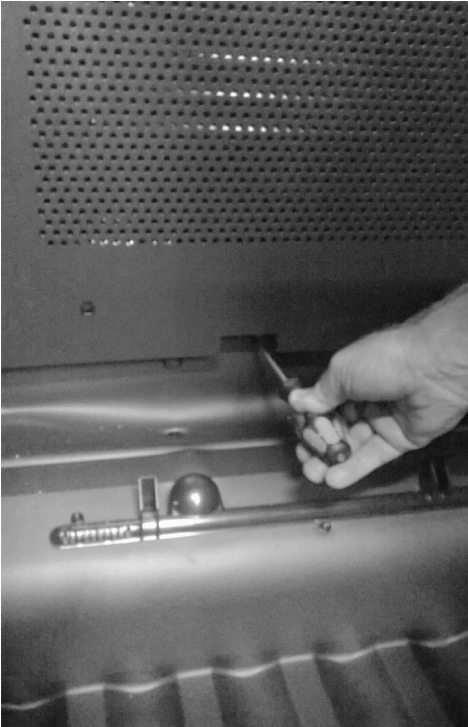
3. Dismantle 2 screws at the bottom ...
