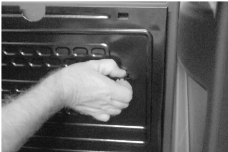
8. Dismantle the 5 evaporator clips. Press to release
