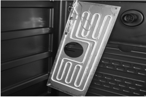
7. Rear of heating element.
