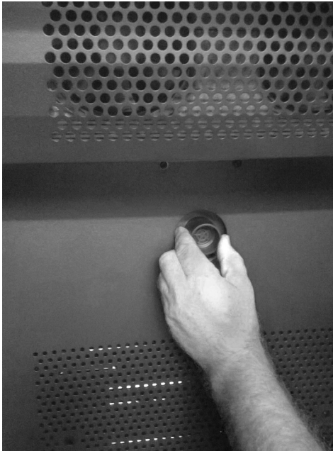
1. Pull out the charcoal filter for replacement.
