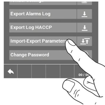
The screen in figure 41 will appear where it is possible to export the PARAM\_EXPORT\_ file. It is possible to save the generated file in the controller's internal memory or on a USB stick.
