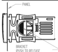
The instruments shall be mounted on vertical panel, in a 29x71 mm hole, and fixed using the special bracket supplied. The temperature range allowed for correct operation is 0÷60 °C. Avoid places subject to strong vibrations, corrosive gases, excessive dirt or humidity. The same recommendations apply to probes. Let air circulate by the cooling holes.
