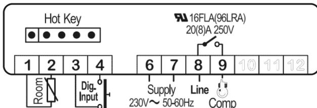
NOTE: The compressor relay is 20(8)A or 8(3)A depending on the model.
