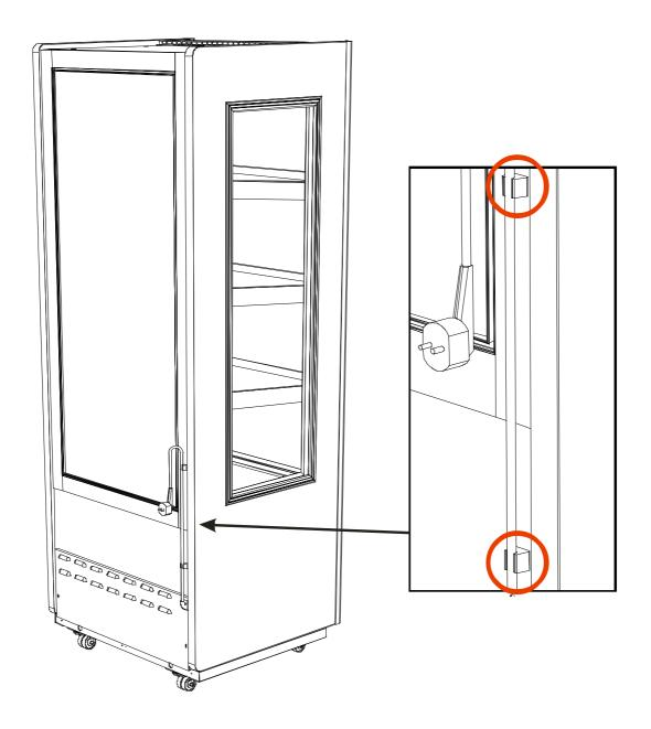
HANG THE POWER CORD TO THE HOOKS DURING CABINET RELOCATION
