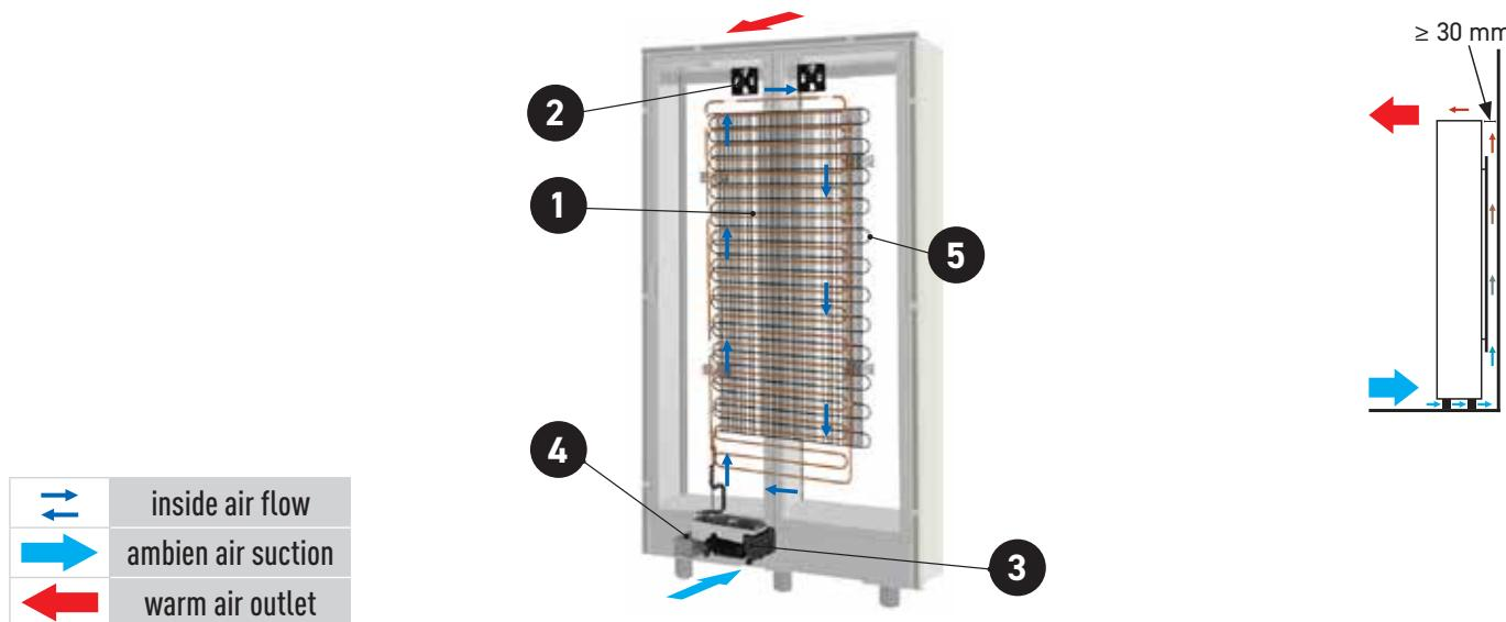
The cooling coil ① and the internal aeration fans ② are placed inside the refrigerated compartment, behind the aluminum back panel. The inverter compressor ③ and the evaporation pan ④ are placed in the lower base. The static condenser ⑤ is installed in the back of the cabinet. The condenser cools down due to convection without the use of fans. Fresh air comes through under the base and rises in the gap between the back of the cabinet and the wall, gets warm and exits from the top.
