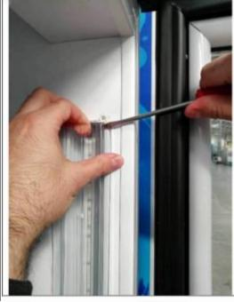
Remove the LED bar by flexing the LED retainer out manually as shown in the figure.
