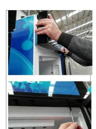
Tighten the upper and lower connection screws of the canopy.
