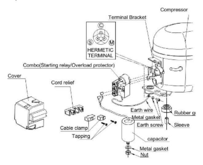
Compressor connection Cubigel model:
