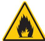
This symbol identifies the refrigerant contained inside of the plant machine is flammable therefore to be posed particular attention in case of damage of the plant or piping and undergoing maintenance.
