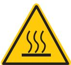
This symbol identifies the danger of hot surfaces in correspondence with the surfaces where it is affixed. In our case this symbol is affixed externally to the cell but refers to the internal surfaces of the latter.
